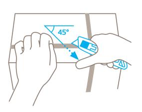
Use the slider to **engage the blade** for cutting. **Pierce** into the cutting material to cut.
