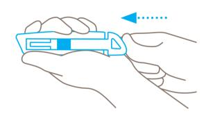
Use the slider to **push** the plastic insert back and out of the handle. Don't pull the insert while holding onto the slider.
