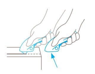
The blade automatically retracts into the handle the moment cutting ceases. Even when the lever is **still being squeezed**.
