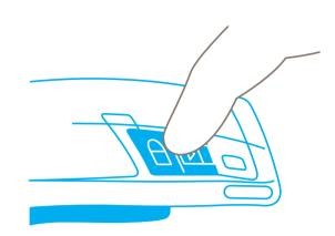
To prevent unintentional blade activation, always **lock the cutter** by pressing downwards on the lock symbol.
