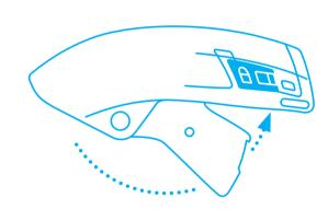
Finally, push the lever back into the handle until you **hear it click into place**.
