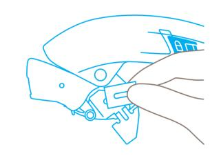
Now you can either **rotate or replace** the blade. Flip the blade cover closed.
