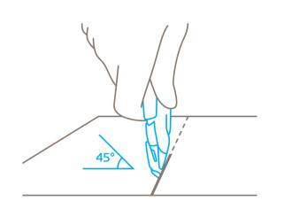
Hold the cutter at a **slight angle** when cutting open cardboard boxes.
