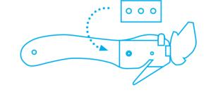
Re-insert the blade **exactly** over the locating lugs and thread.
