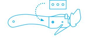
Re-insert the blade **exactly** over the locating lugs and thread.
