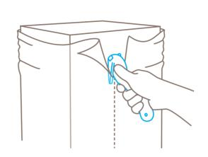
Use the pointed nose to **pierce** the material to be cut. You can also use it to guide the cut.
