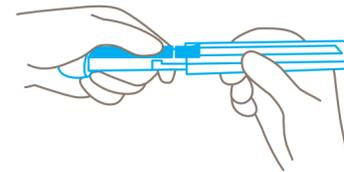
When the slider and blade leave the handle, position your **index finger under the blue blade holder** to hold it tight.
