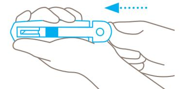
Make sure you position the blade **exactly over the locating lugs**, close the blade holder upwards. **Attention:** Never hold your hand in front of the blade exit!
