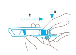
**Press** the blade change button and remove the plastic insert from the rear of the handle.
