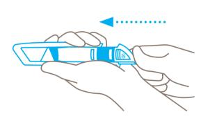
Close the blade cover and push the plastic insert back into the handle until the blade change button audibly clicks.
