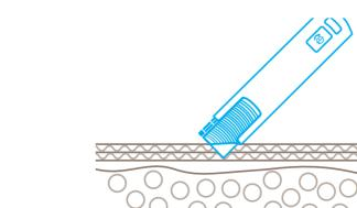
Following cutting, the blade immediately retracts into the handle. Condition: you have released hold of the slider.
