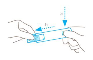
Press the blade change button downwards and **at the same time** pull out the slider all the way from the front.
