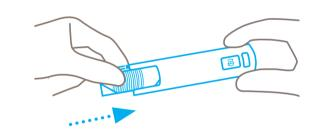
Finally, re-insert the slider and blade **fully** into the handle.
