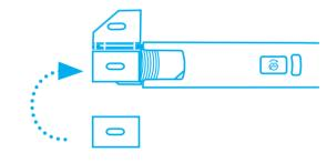
Reverse or replace the blade. Make sure you position the blade **exactly** over the location lobes. Close the cover.
