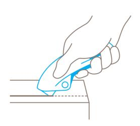
To engage the blade, unlock the cutter and **squeeze the lever**. Now you can cut.
