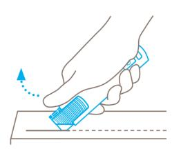
Always remove your **thumb from the slider** to For best results, cut plastic strapping band ensure automatic blade retraction.
