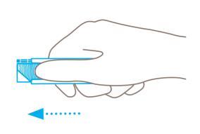
Use the slider to **engage the blade** for cutting.
