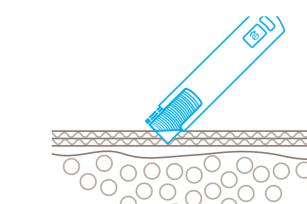
Following cutting, the blade immediately retracts into the handle. Condition: you have released hold of the slider.
