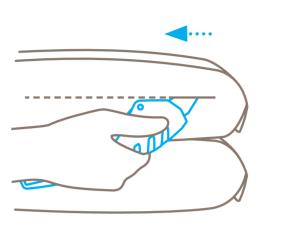
... and **cut into** the material (e.g. bag). **Important**: Never cut towards the body. After cutting, **releasing the lever** retracts the blade.
