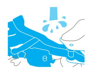
Remove the blade **before** cleaning! Use compressed air, water, alcohol or acetone depending on the type of dirt.
