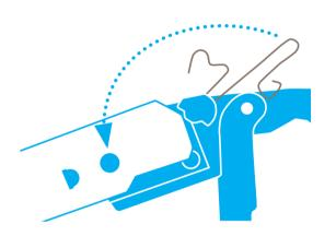
**Lock the spring** and swivel the **lever** back into the handle until it automatically **locks** into place. Unlock the lever and press once to test.
