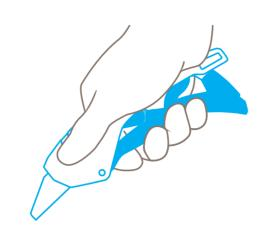
The **blade** can now be **released** using the lever ...
