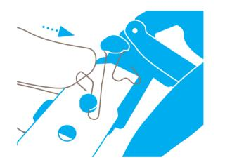
Release the spring from the groove by applying **light pressure** and by pressing it to the side. Change the blade and put the replacement **precisely** on the location lobes.
