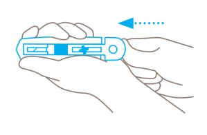
Use the slider to **push** the plastic insert back and out of the handle. Don't pull the insert while holding onto the slider. When the slider and blade exits the handle, position your **index finger under the black blade holder** to hold it tight.
