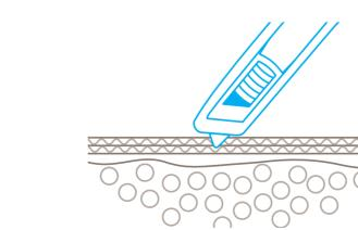
Following cutting, the blade immediately retracts into the handle. Condition: you have released hold of the slider.
