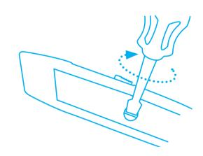
Make sure you place the blade **exactly** on the Place the upper half of the handle back on the lower half and fasten the screws **tightly** by hand.
