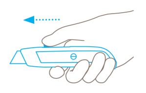
**Extend** the blade by moving the slider forward.
