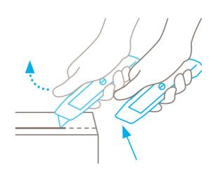
Following cutting, the blade immediately retracts into the handle. Condition: you have released hold of the slider.
