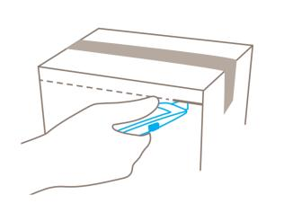
Always remove your **thumb from the slider** to ensure automatic blade retraction.
