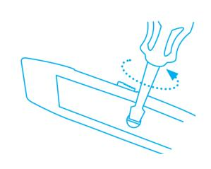
**Unscrew** the handle and remove the upper half of the handle.
