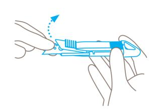
Take hold of the blade and nudge the blade cover open: either **rotate or replace** the blade.
