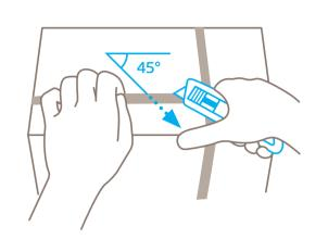
For best results, cut plastic strapping band **diagonally** (at a 45° angle).
