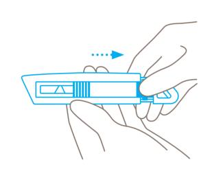
Press the blade-change button and **pull out the plastic insert**.
