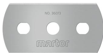
INDUSTRIAL BLADE NO. 36013 from MARTOR is a high-quality blade made of steel. It is very sharp and has four cutting edges that can be used one after the other for an extra long service life. The blade is 43.4 mm long, 22 mm wide and 0.13 mm thick.
